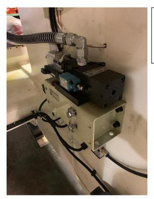
Fast acting hydraulic overload pump (H.O.L.P) prevents hydraulic overload due to a bad set-up or during parts stacking. Adjusted in our facility with our precision load-cell, the hydraulic overload is tested several times prior shipment to prevent any bad application.
