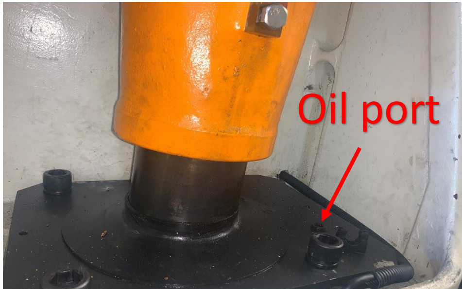
FIGURE 7.4.9.4 ADJUSTMENT SCREW OIL PORT INLET
